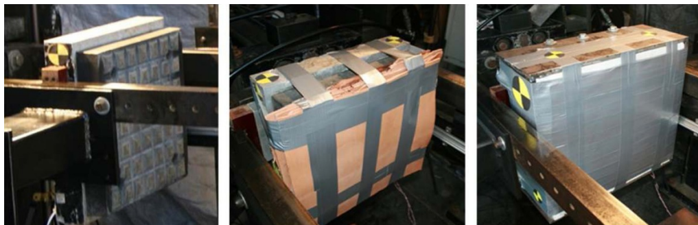
Fig. 7. Impact materials from left to right: urethane, leather, confined sand.
