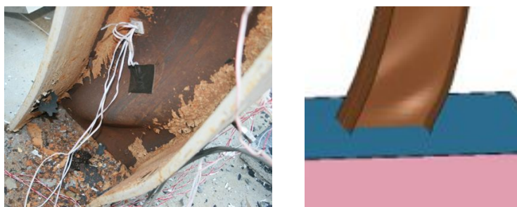
Figure 11: Local buckling comparisons for Test SA-11.
