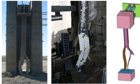
Figure 13: Field, Simulator, and FEM comparisons for column without cladding.
