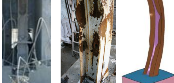
Figure 12: Field, Simulator, and FEM comparisons for column with cladding.
