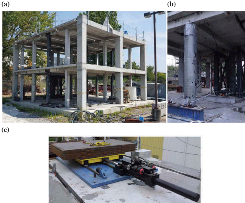
Figure 1. Full-scale, two-story two-bay non-ductile RC test frames: (a) four identical full-scale test frames; (b) FRP jacketed column in the retrofitted test frame; (c) hydraulic linear shaker on the roof of the RC test frames [Shin et al. , 2016].
