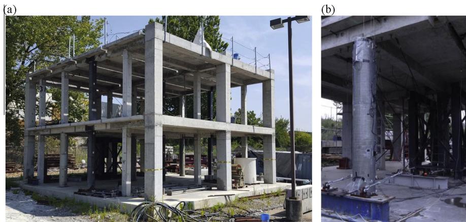
Fig. 3. Full-scale, 2-story 2-bay non-ductile RC test frames: (a) Four identical full-scale test frames; (b) FRP jacketed column in retrofitted test frame.
