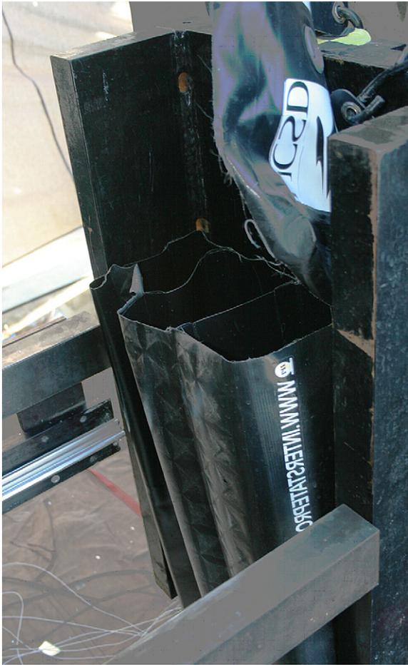
Fig. 5. Photo of typical vertical internal baffles used to control water flow within the bladders and provide additional structural reinforcement.
