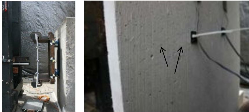
Figure 10: Test 14 posttest damage from side (left) and back (right).
